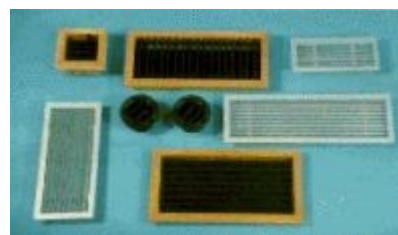
The pictures show the use of the air distribution grills, their shape and some of the possible installations. As the cold air is heavier than warm air, the cold air falls therefore the cooled air should be dispersed across the deck head or at least upwards. This is achievable also by realigning the grill blades. The air grill has also a high impact on the inside decor.
