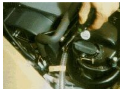
Picture 19: The in and out hoses are then connected to the air-conditioner, taking care to respect the indications of the water flow direction. Great care must be taken in installing the Jubilee clips.
