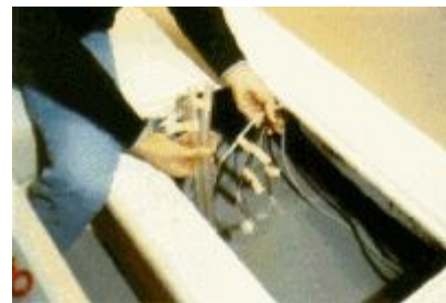
Picture 12: The space under the seat (sofa) is where the unit will be installed. In this space we install the two sea water hoses (in and out) and the electrical connecting cables. The sea water out through hull fitting must be drilled as low as possible on the water line in order to reduce to a minimum any noise from the falling water. (see drawing 6)
