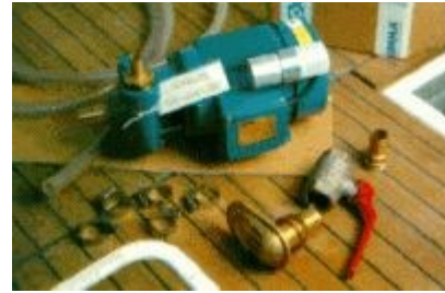
Picture 8: The picture shows the components of the sea water circuit: A through hull "scoop" type intake, a manual valve, a centrifugal pump, different diameters hoses, and jubilee clips of different sizes.
