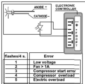
The Danfoss BD35 and BD50 compressors have their own fault diagnostic allowing easy fault finding. The fault code will only be shown when the compressor fails to start or stops.
