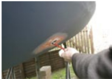
Wires and tubes are fed up through the hole so the unit can be secured. This is best achieved as a two-person job - one to hold the unit in position and one to tighten the nut from inside
