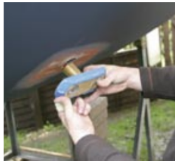
Care should be taken to ensure the unit is aligned fore-and-aft to minimise drag
