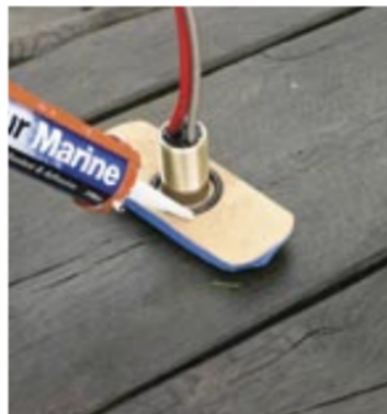
Underwater adhesive-sealant was applied to the back of the unit to ensure a watertight fit
